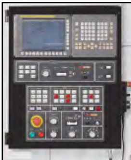
Fanuc 0iTF control with 10,4" LCD display and Manual Guide i
