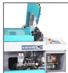
Hydr. unit and electrical panel
