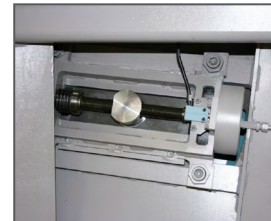
Blade tensioning KTECH via electro-mechanical system, CNC-controlled
