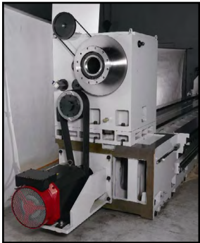
Rigid headstock built-in with gear box
