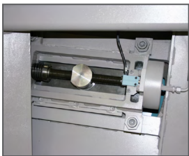
Blade tensioning KTECH via electro-mechanical system, CNC-controlled
