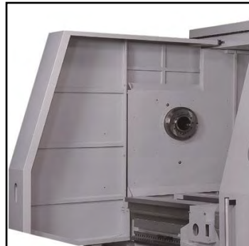
Well-protected chuck guard with interlock switch
