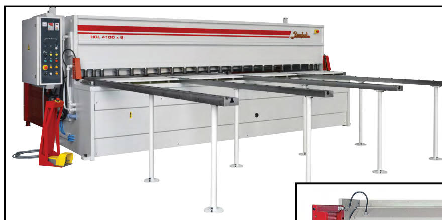
Pneumatic sheetcatcher type B with ball spindles
