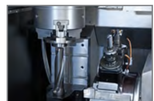
Multi-functional plate, supports long drilling tools
