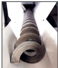
Mot. chips conveyor, hydraulically driven
