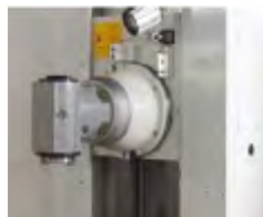
Right angle milling head
