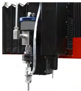
Equipment for pre-drilling of fragile and multi-laminated composites. Possible to mount different drill bit diameters.
