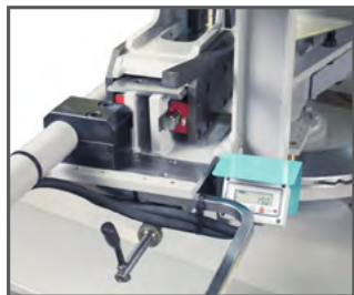
Digital display showing angle of sawframe
