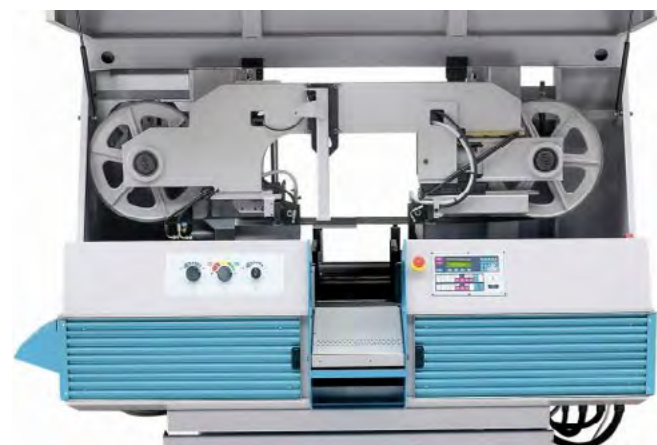
Special double section of saw frame
