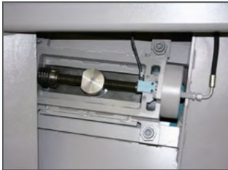
Blade tensioning KTECH via electro-mechanical system, CNC-controlled
