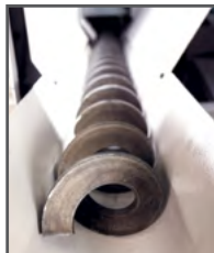
Mot. chips conveyor, hydraulically driven
