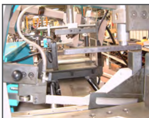
Hydr. device for bundle cutting
