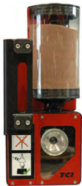
Automatic abrasive regulator. Stops automatically when the abrasive has been used up.
