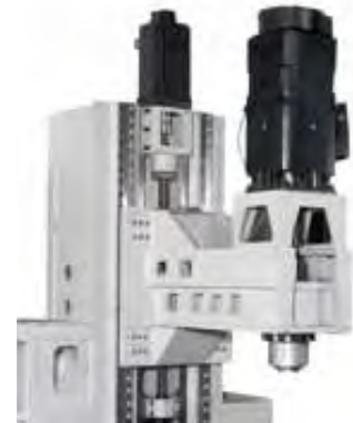
12.000 RPM in-line spindle
