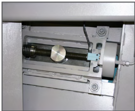
Blade tensioning KTECH via electro-mechanical system, CNC-controlled
