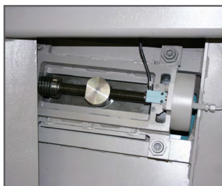
Blade tensioning KTECH via electro-mechanical system, CNC-controlled
