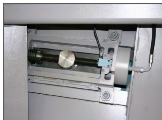
Blade tensioning KTECH via electro-mechanical system, CNC-controlled
