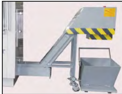
Chip conveyor can easily be retrofitted
