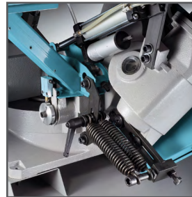
Springs for perfect balance of the saw frame
