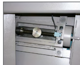
Blade tensioning KTECH via electro-mechanical system, CNC-controlled
