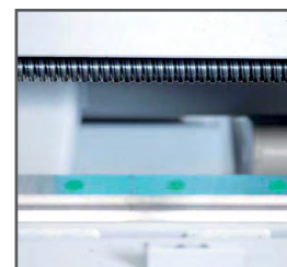
Screw feeder in all automatic NC bandsaws
