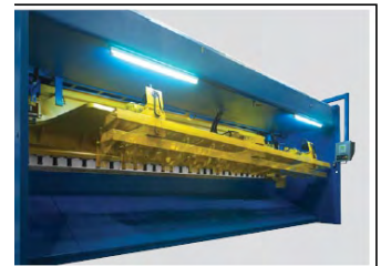
Automatic swing-up for longer cuts
