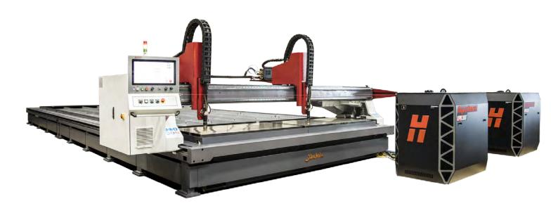
This plasma cutter is ideal for larger productions in plasma cutting, because it is possible to mount multiple plasma cutting heads combined with oxygen cutting heads. Up to 4 plasma cutting heads or up to 8 oxygen cutting heads. (Max 8 Cutting heads total)
