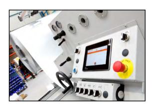
Ekicontrol coil processing line type COMPACT is a slitting and cut-to-length line with straightener, all placed on the same common base. Electric equipment and touch screen for programming are integrated into the structure of the machine. The machines are 100% European using only European components of the highest quality. The line has a 10-ton loading capacity of coil.
