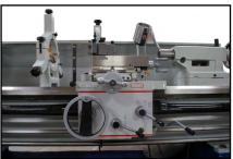
**Type GH-1860** precision lathe with hardened and ground bedways and gears. With Camlock spindle nose for quick change of chucks, foot brake and halogen work lamp. Cast-iron stand. Jog button switch for easy spindle speed selection. Gap bed allows larger diameter work. Gear runs in oil bath. Practical central location of controls.
