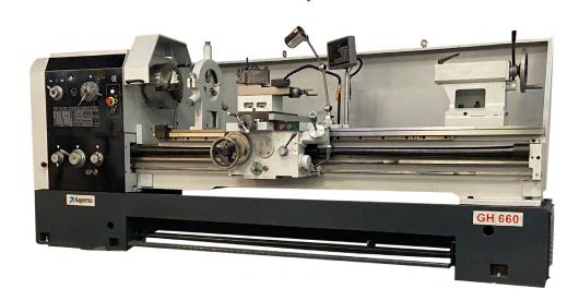
**Type GH 660** precision lathe with hardened and ground bedways and gears. With Camlock spindle nose for quick change of chucks, foot brake and halogen work lamp. Cast-iron stand. Jog button switch for easy spindle speed selection. Gap bed allows larger diameter work. Gear runs in oil bath. Practical central location of controls.
