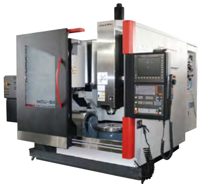
Microcut bearbn.center MCU-5X 5-akset, Heidenhain TNC640 styring, 15000 o/min.
