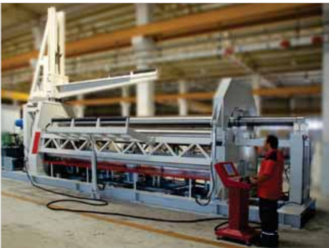
Pre-stressed plate bending machine for pipe production
