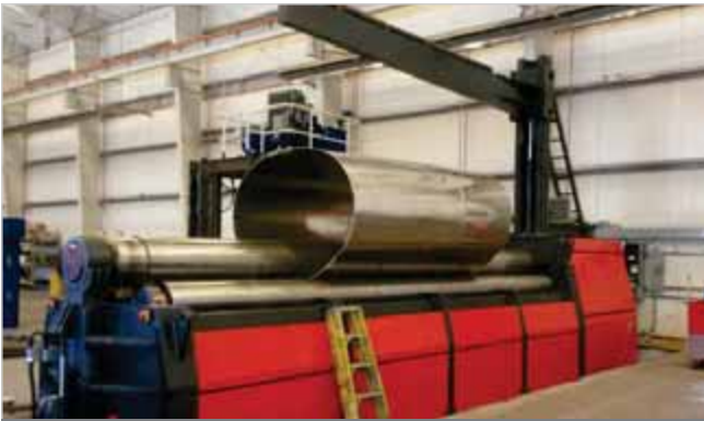
AHS 7700 x 9/12 CNC Four Rolls Hydraulic Plate Bending Machine
