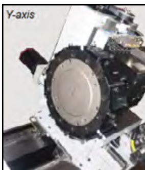
Y-axis enables diverse and off-center machining for complicated parts
