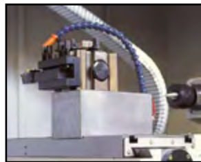
Quick change tool post fitted
