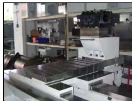
Twin prismatic guideways in inverted "V" for the cross slide
