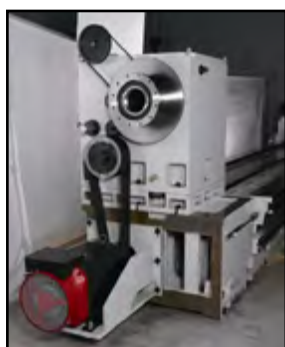
Rigid headstock built-in with gear box
