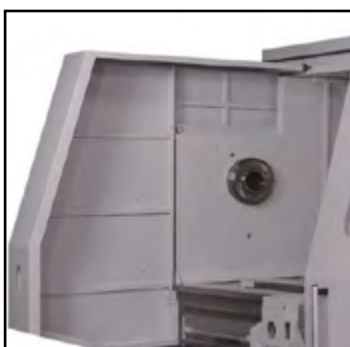
Well-protected chuck guard with interlock switch
