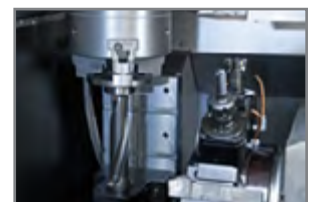
Multi-functional plate, supports long drilling tools
