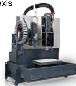
Machine base made from vibration damping polymer concrete
