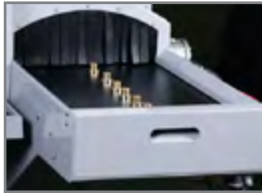
Part catcher conveyor
