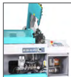
Hydr. unit and electrical panel
