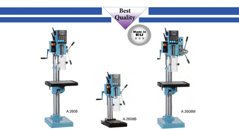
**ARBOGA A2608** has a drilling capacity of 25mm. The gearbox is built according to our experienced methods for highest possible torque. Helical gears combined with steel gears against reinforced fibre gears in the main gear box ensure higher operation efficiency, a more powerful drive mechanism and smooth operation. Both the drill head and the table arm are adjustable 360° around the column and can be raised and lowered.
