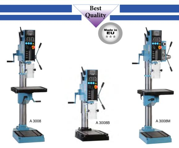
**ARBOGA A3008** has a drilling capacity of 30mm. Helical gears combined with steel gears against reinforced fibre gears in the main gear box ensures higher operation efficiency, a powerful drive mechanism and smooth operation. A 3008 is standard-equipped with a handreversing switch. Both the drill head and the table arm are adjustable 360° around the column and can be raised and lowered.
