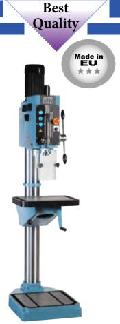
**ARBOGA A4008** has a drilling capacity of 40mm. The gear box is built according to our experienced methods for highest possible torque. The drill head is fixed on top of the column. The table arm is adjustable 360° around the column and can be raised and lowered.
