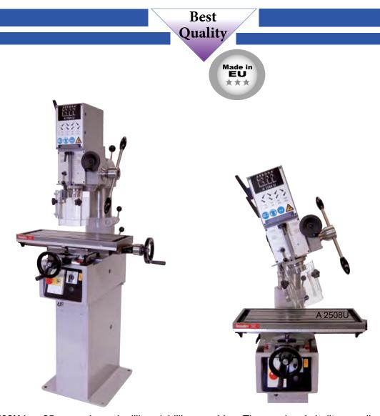
**ARBOGA A2508U** is a 25 mm universal milling- / drilling machine. The gearbox is built according to our experienced methods for highest possible torque.
