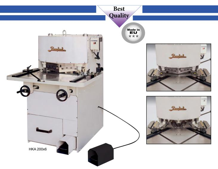
Hydraulic corner notcher type HKA is build with an extremely solid frame, large and functional working table and an effective notching head. Adjusting of the cutting angle is done using two hand wheels, which ensure easy and accurate operation. Type HKA is equipped with automatic cutting gap adjustment for all thicknesses. The machine is designed with square guides, scales and angle gauge.
