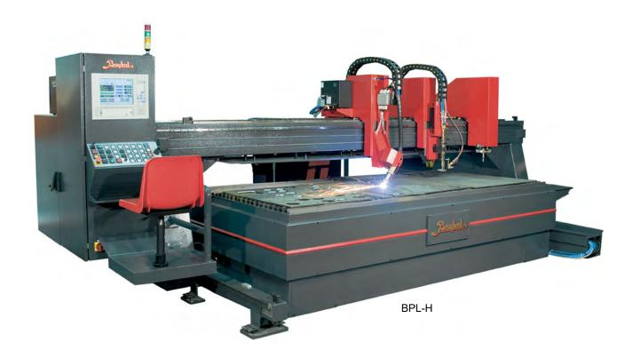
This plasma cutter is ideal for larger productions in plasma cutting, because it is possible to mount multiple plasma cutting heads combined with oxygen cutting heads. Up to 4 plasma cutting heads or up to 8 oxygen cutting heads. (Max 8 Cutting heads total)
