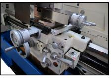
**Type GH-1640A** precision lathe with hardened and grounded bedways and gears. With Camlock spindle nose for quick change of chucks, foot brake and halogen work lamp. Cast-iron stand. Jog button switch for easy spindle speed selection. Gap bed allows larger diameter work. Gear runs in oil bath. Practical central location of controls.
