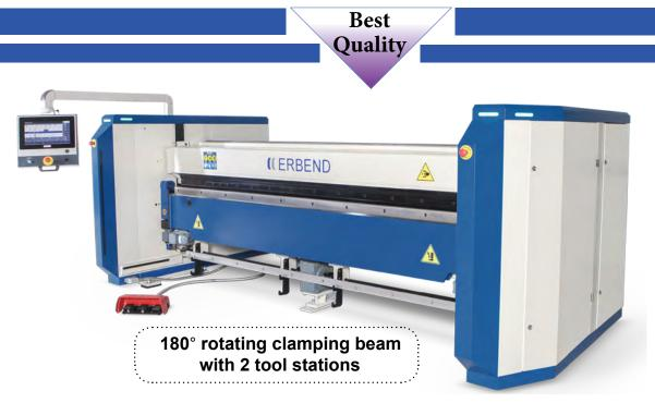
Erbend CNC motorised folding machine type MFD is a sturdy machine with high speed and high flexibility with 180° rotating clamping beam with 2 tool stations. MFD is an extremely versatile folding machine, able to bend many different profiles, boxes etc. by means of various tools, which are easy exchangeable. You can design and produce your items in a few minutes by means of the user friendly control.
