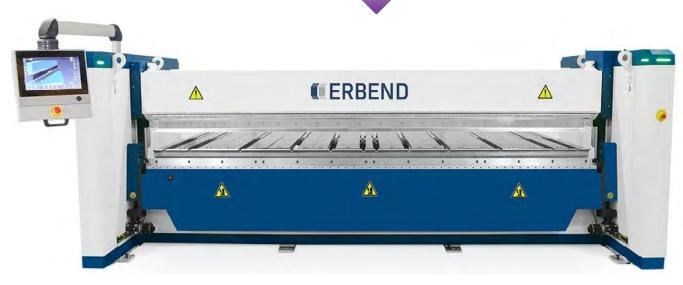
Erbend CNC servo motorised folding machine type SFA is a sturdy machine with high speed and high flexibility. SFA is an extremely versatile folding machine, able to bend many different profiles, boxes, etc. by means of various tools, which are easy exchangeable. Thanks to 350 mm Z-axis stroke and 170 mm high goat foot tools you can make deeper flange, box bendings. You can design and produce your items in a few minutes by means of the user friendly control.
