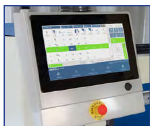
Erbend 2D / 3D CNC styring
