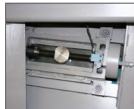
Blade tensioning KTECH via electro-mechanical system, CNC-controlled
