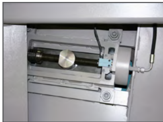
Blade tensioning KTECH via electro-mechanical system, CNC-controlled
