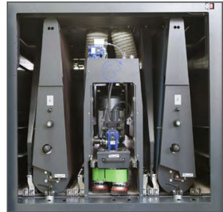
Roller unit Ø250 / Tangential brushes system / planetary system / Electronic grit set
