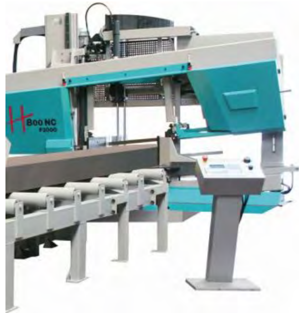
KS 802 NC with roller table - various roller tables are available, also in motorised and vertical versions
