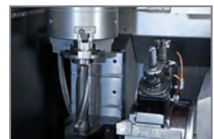
Multi-functional plate, supports long drilling tools
