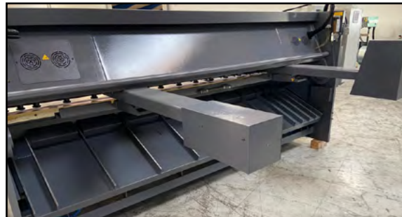
Pneumatic sheet catcher type Universal
