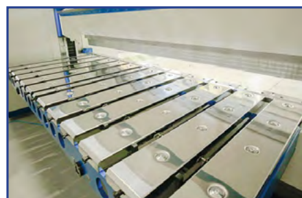
Stainless steel back gauge table covers
