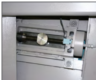
Blade tensioning KTECH via electro-mechanical system, CNC-controlled
