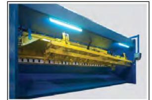
Automatic swing-up for longer cuts
