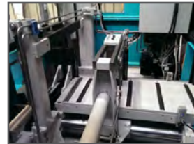
SMART feeder with built-in supporting table
