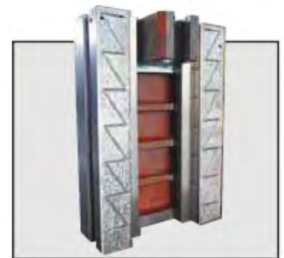
Guideway - box-way structure
