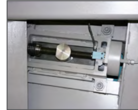
Blade tensioning KTECH via electro-mechanical system, CNC-controlled
