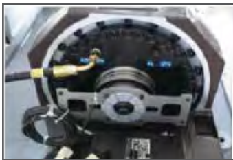
Angle encoder - High-precision angle encoder fits on A-axis and C-axis.
