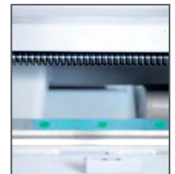
Screw feeder - in the automatic NC bandsaws the movement of the feeder is via a recirculating ballscrew and gear motor controlled by an inverter
