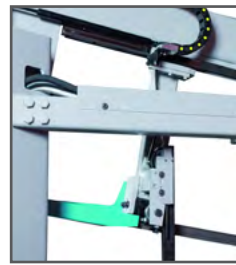
Mobile blade guide automatically kept in contact with the cutting point.
