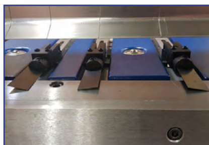
Solid lower beam tool and feather grooves
