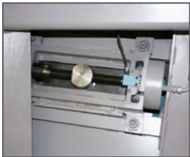
Blade tensioning KTECH via electro-mechanical system, CNC-controlled
