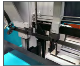
Double vices before and after the band blade, ensuring a perfect clamping of the bar during operation
