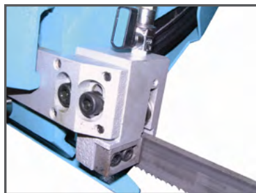
Blade guides with hard metal pads
