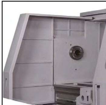
Well-protected chuck guard with interlock switch
