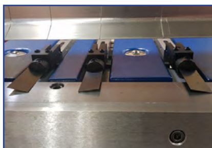
Solid lower beam tool and feather grooves
