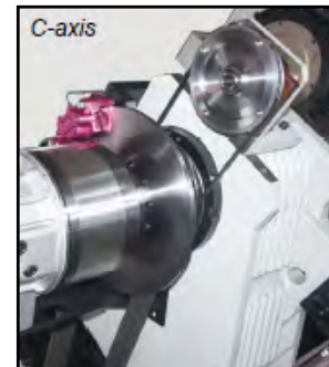
C-axis with braking system provides spindle angle indexing & superior performance
