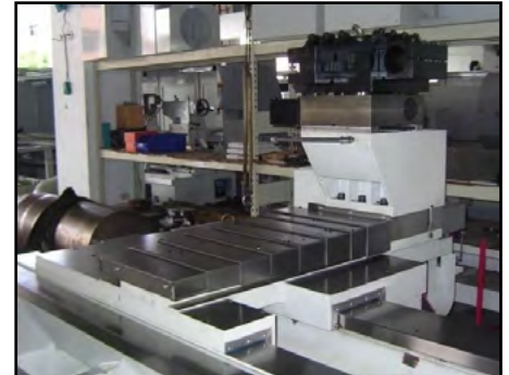
Twin prismatic guideways in inverted "V" for the cross slide
