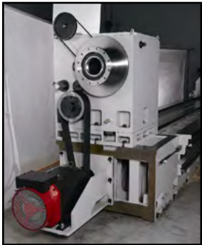
Rigid headstock built-in with gear box
