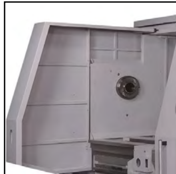
Well-protected chuck guard with interlock switch
