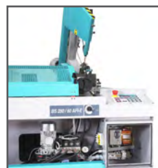
Hydr. unit and electrical panel
