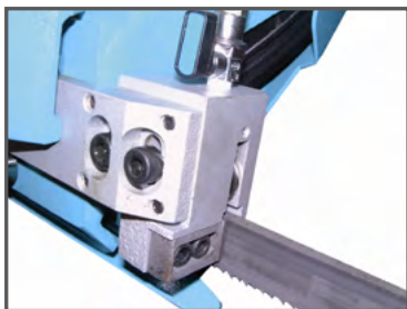
Blade guides with hard metal pads
