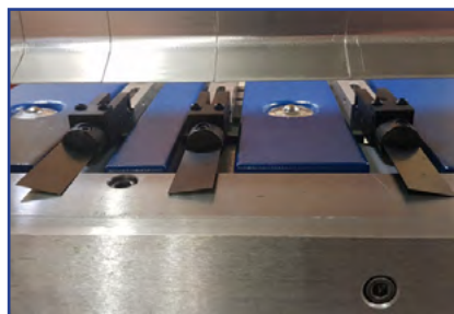
Solid lower beam tool and feather grooves
