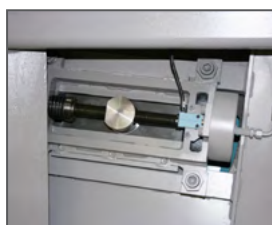
Blade tensioning KTECH via electro-mechanical system, CNC-controlled
