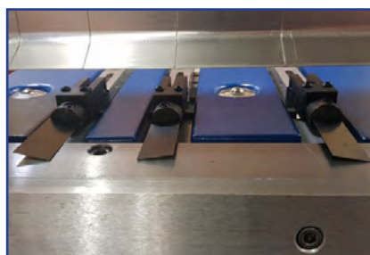
Solid lower beam tool and feather grooves
