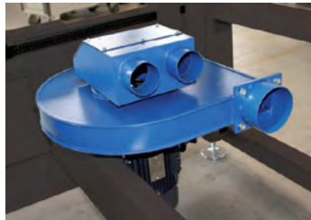
Internal vacuum fan (setting variable inverter)
