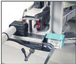
Digital display showing angle of sawframe
