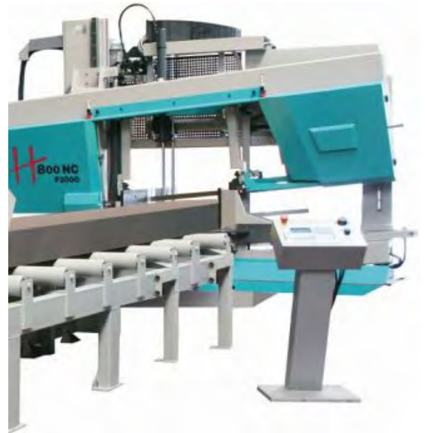
KS 802 NC with roller table - various roller tables are available, also in motorised and vertical versions
