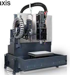
Machine base made from vibration damping polymer concrete
