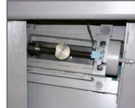
Blade tensioning KTECH via electro-mechanical system, CNC-controlled
