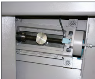
Blade tensioning KTECH via electro-mechanical system, CNC-controlled
