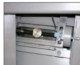
Blade tensioning KTECH via electro- mechanical system, CNC-controlled
