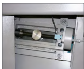
Blade tensioning KTECH via electro-mechanical system, CNC-controlled
