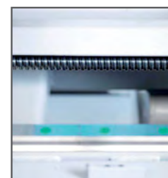
Screw feeder - in the automatic NC bandsaws the movement of the feeder is via a re-circulating ballscrew and gear motor controlled by an inverter
