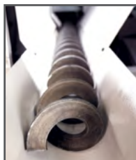
Mot. chips conveyor, hydraulically driven
