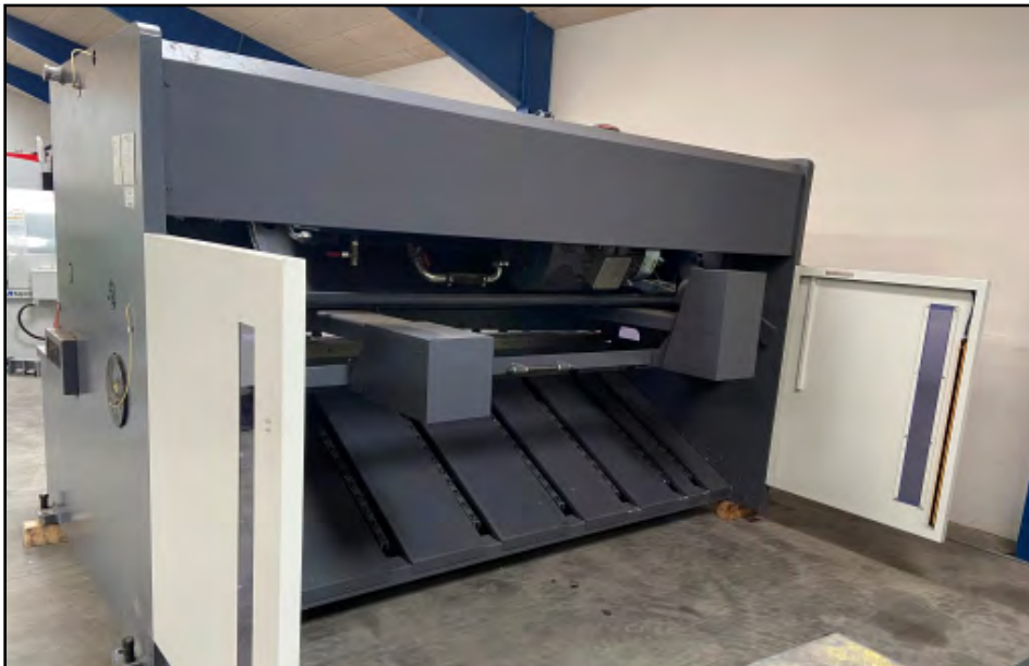
Pneumatic sheet catcher type D
