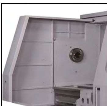
Well-protected chuck guard with interlock switch
