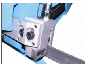
Blade guides with hard metal pads
