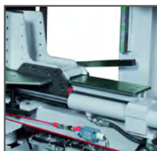
Safety wire detecting obstacles
