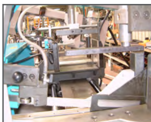
Hydr. device for bundle cutting
