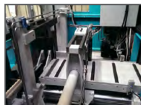
SMART feeder with built-in supporting table
