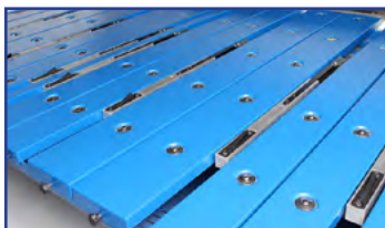
1500-2000-3000-4000 mm mot. back gauge + support
