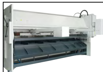
Pneumatic sheetcatcher type universal
