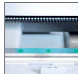
Screw feeder in all automatic NC bandsaws
