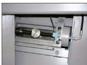
Blade tensioning KTECH via electro-mechanical system, CNC-controlled
