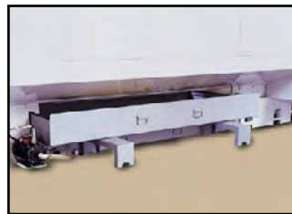
Easy retrofit chip conveyor
