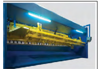
Automatic swing-up for longer cuts
