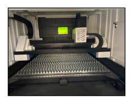
Senfeng 1313N fiber laser is a modern laser in a compact and elegant design. SF1313N is delivered with a generator fom either Maxphotonics, IPG or Raycus, 1,5-6 kW.
