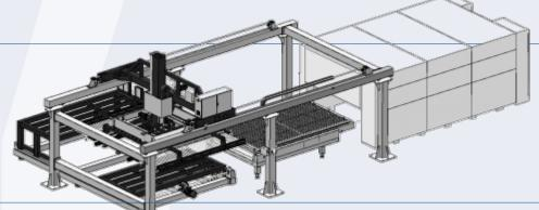
2.2 Cartesian coordinates 500kg loading and unloading manipulator are adopted, with linear guide rails, and full servo drive. The translational running speed is adjustable from 10-50m/min. The lifting speed is 5-10m/min, which is infinitely adjustable. The repeated positioning accuracy of the loading and unloading manipulator  $\pm$  1.5mm.
